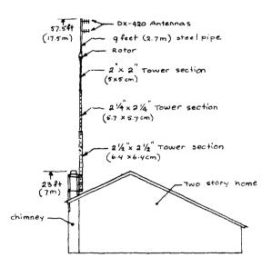
fig. 1. Tower and antenna assembly measures 57.5 feet (17.5 meters) from ground.
